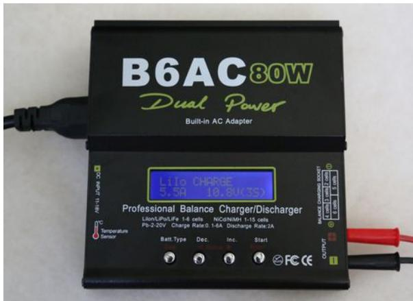
6. Set the desired charging current. The battery for a maximum charging current of 10A is approved. However, we strongly recommend a charging current of 5A – 6A.
